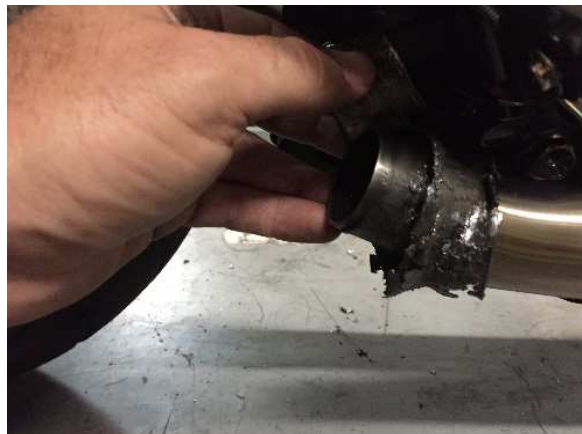
Unwrap broken gasket and remove.
