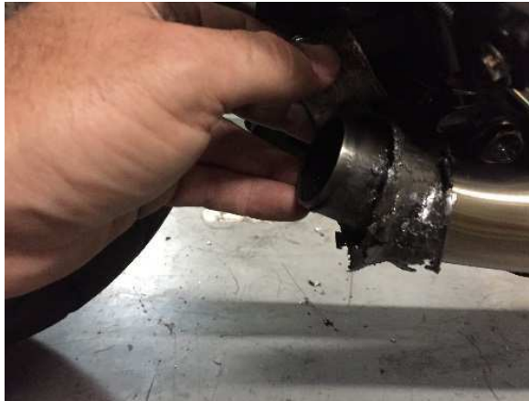
Unwrap broken gasket
