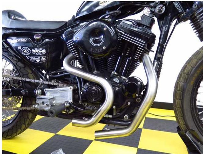
4. Install support bar racket onto the tab mounted on the exhaust. Leave it loose so you have plenty of adjustment range.
