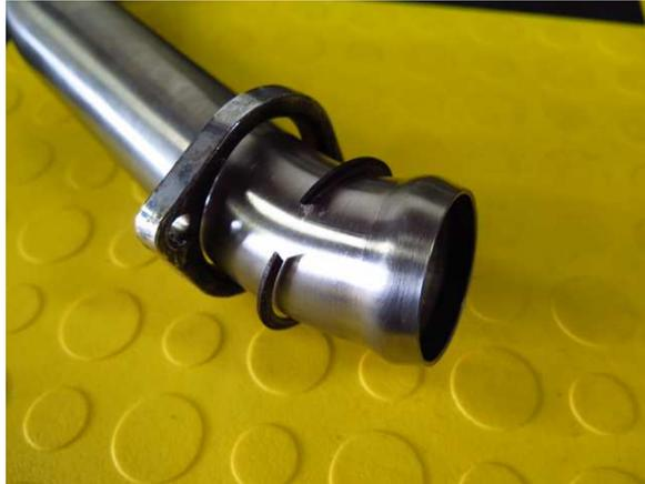
3. Begin by loosely installing the headers in the cylinder head and start the flange bolts, *don't tighten them yet.*
