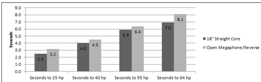
Like a race, the first to the finish is the winner. These results show that not only did our muffler get to a higher overall power, but it did so significantly more quickly. Note that in the second graph not only is there a time differential, but the open header never reaches the same total horsepower as the muffler does.
